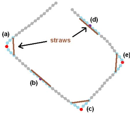
**Figure 2:** An example of “straws” in a stroke. The points (a-e) all have a window of  $\pm 3$  points. the distance at endpoints at these windows forms a straw, with the shortest straws being at points (a), (c), and (e). These points are considered corners. Points (b) and (d) have straws that are close to the median straw length, so these points are not initial corner candidates.
