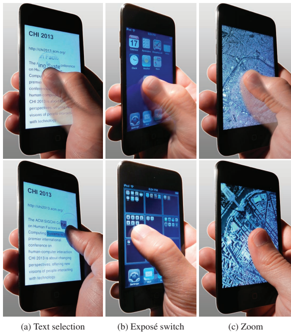
Figure 12: Application prototypes using the ThumbRock. Top row shows the ThumbRock being performed and bottom row the subsequent action.
